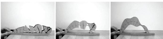
Figure 14. Post tension erection prototype. This method negates the need for formwork.
